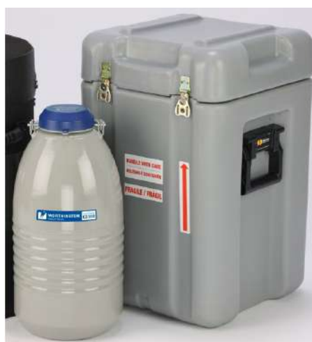
Figure 10: Dry Shipper with Shipping case and labelling
