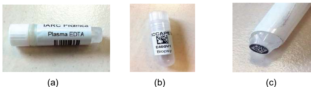
Figure 6: Pre-labelled cryogenic specimen storage container. (a) Printed linear barcode, (b) Printed two-dimensional barcode, and (c) pre-labelled tube with two-dimensional barcode.
